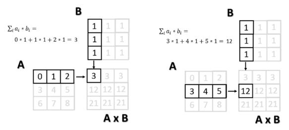
Figure 3-2. Calculating matrix elements as a result of a matrix product
