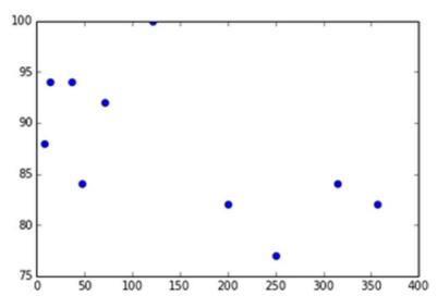
*Figure 10-16.* The trend of the maximum humidity function with respect to the distance from the sea
