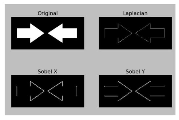
*Figure 14-16. The result from the edge detection applied to the blackandwhite.jpg image*
