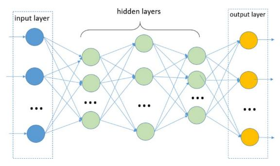
*Figure 9-2.* A schematization of how a generic artificial neural network is structured
