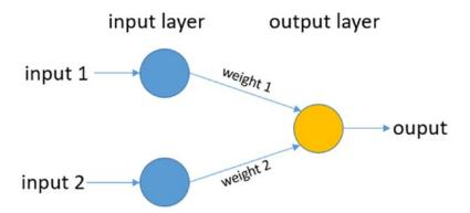
Figure 9-3. The Single Layer Perceptron (SLP) architecture
