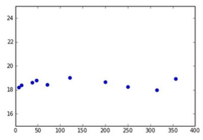
*Figure 10-14.* The minimum temperatures appear to be independent of the distance from the sea
