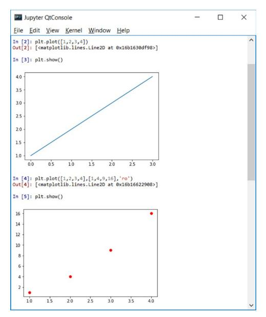
**Figure 7-7.** The pairs of (x,y) values are represented in the plot by red circles
