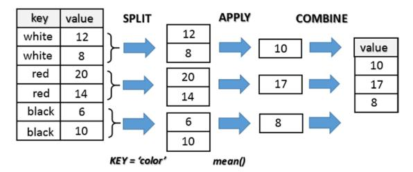
Figure 6-1. The split-apply-combine mechanism
