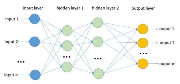
Figure 9-6. The Multi Layer Perceptron (MLP) architecture
