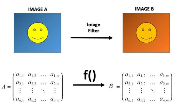
*Figure 14-9.* A representation of the image filters that are the basis of image analysis
